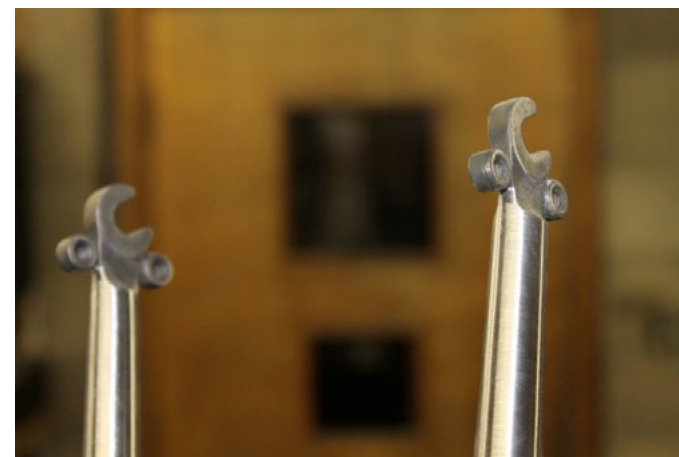
After sanding, the dropouts appear perfectly blended into the fork blades.
