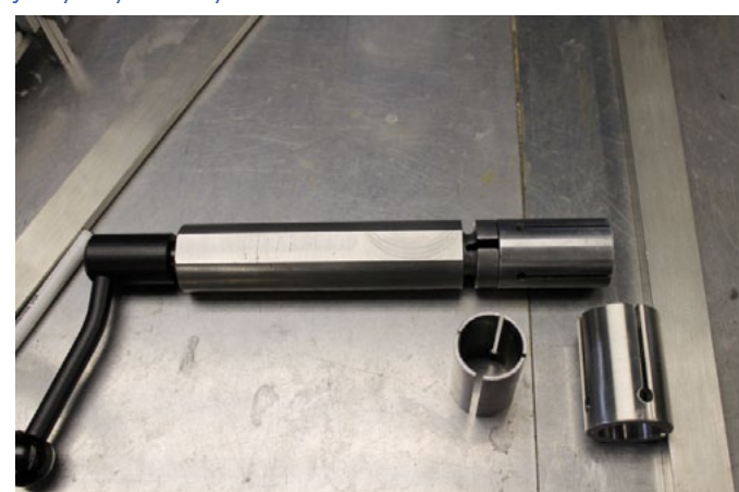
Herbie Helm's own design lug vice, for holding lugs firmly while they are filed.
