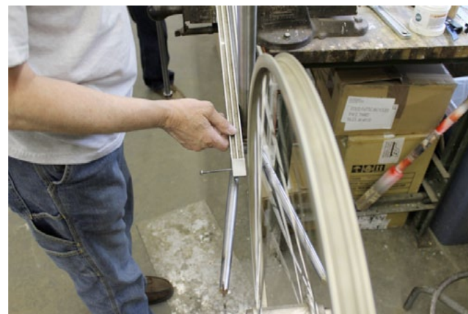
A straight edge tool is used with a wheel for a final alignment check.
