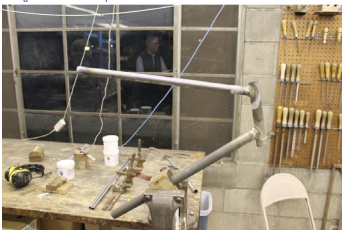
Part of the frame ready to be brazed.
