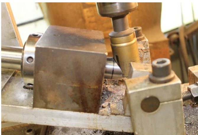
The tube is held in a collet on the milling machine.
