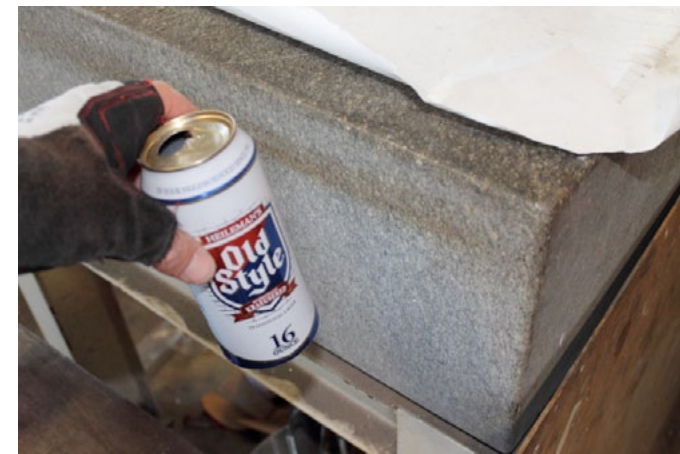
Granite surface table - the beer can is for scale.
