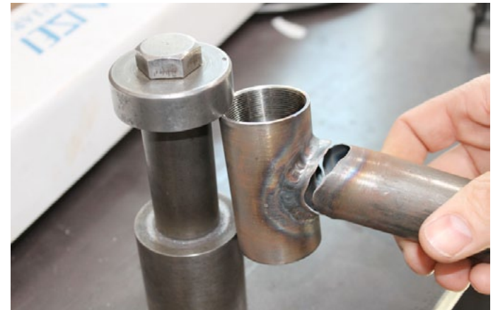
The welded or brazed joints are then tested by inserting a bar and levered on. A break on the weld = failure. Above the weld = good join.
