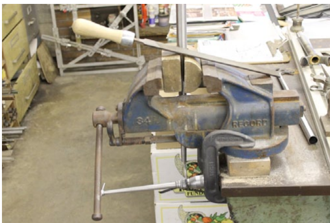
Filing an 8 degree mitre in the chainstay
