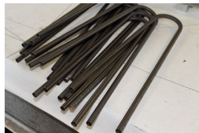
4130 cro-mo tubing for wishbone seatstay rear ends.
