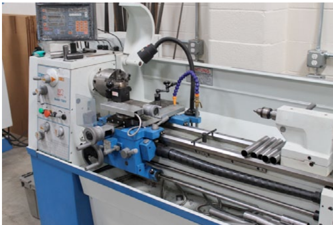
Head tubes, steerers and crown race seats are cut on this lathe.
