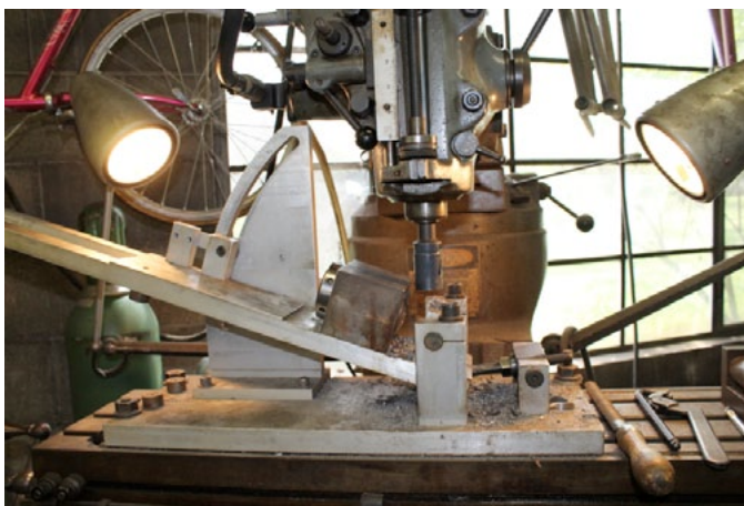
Tube held in mitring fixture on the Bridgeport milling machine.
