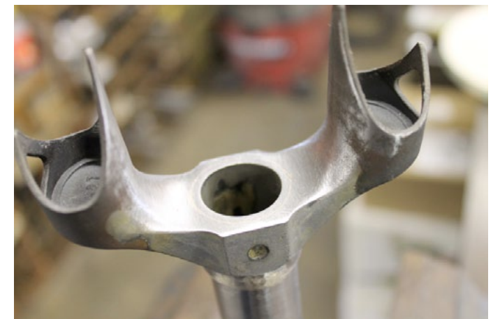
Excess silver braze and steerer material is filed away.
