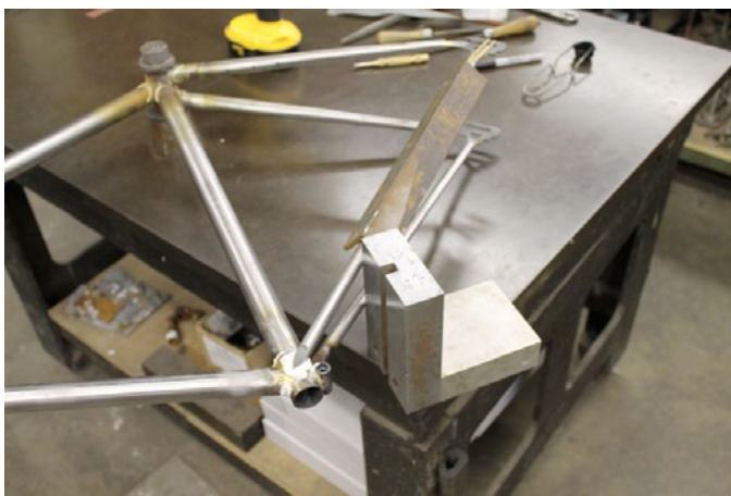
Pre-braze set up on the alignment table.
