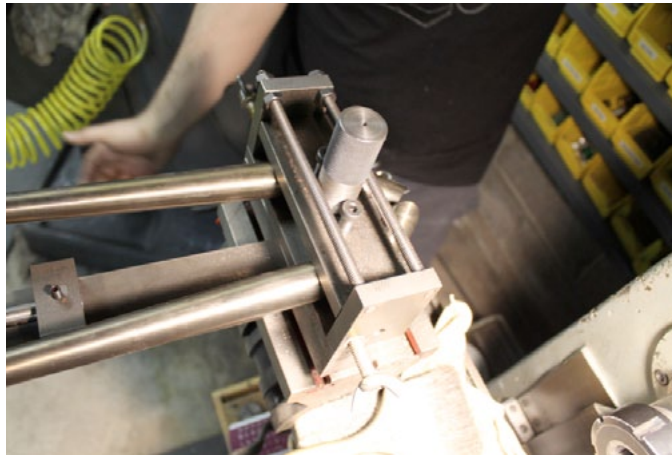
The tops of the blades are clamped down to keep the blades in phase.
