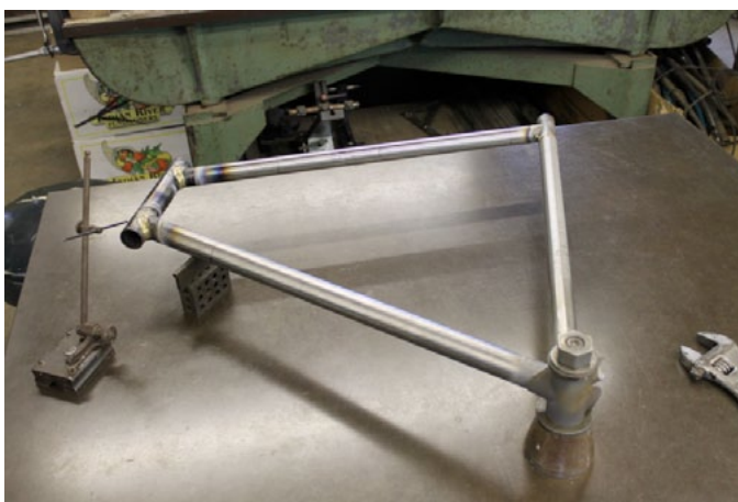
Checking the post braze frame alignment with a surface gauge on the table.
