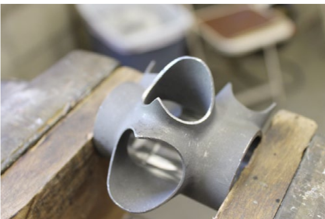
Bottom bracket: cleaning up the edges and putting a point on the tip. We used a Swiss file, and Doug showed us some neat tricks.
