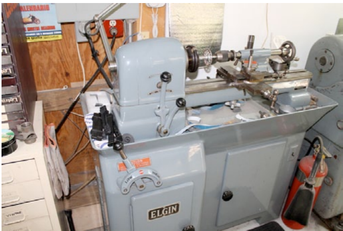
A lathe with constantly variable speed.
