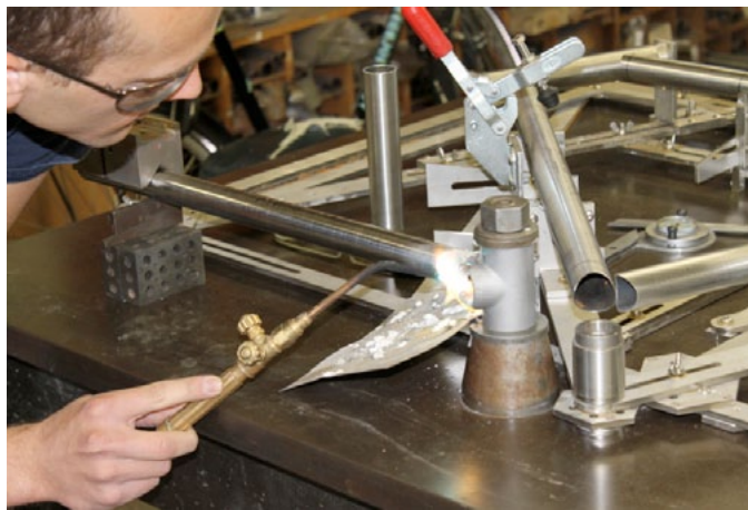
Herbie tacks a seat tube into a bottom bracket shell
